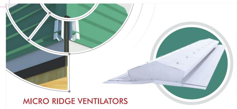
ARV micro ridge vents are aesthetically appealing, and are an extremely efficient means of ventilating metal roofs. Each unit is manufactured in 10 feet lengths and can be installed as a single unit or can be butted together to form a continuous run. By lapping the furnished joint covers over the top of the butted joints in a continuous run, the vent has the appearance of a single unit.
